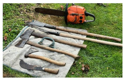
Toni's hedge laying tools. The small axe was forged to Toni's specification at an ironmongers in Kineton. Toni wanted a lightweight axe to make fine cuts that are difficult to do with a heavier axe.
